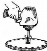
Drilling the holes in the centralizer
