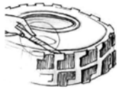
Cut out a section of rubber
